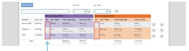
Check the corresponding box if the Excipient is used for Wet Granulation (WG) or Direct Compression (DC). Check both boxes if the Excipient can be used in both manufacturing methods. The color coding provides a quick overview.
