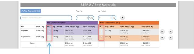
Check the corresponding box if the API is used for Wet Granulation (WG) or Direct Compression (DC). Check both boxes if the API can be used in both manufacturing methods. The color coding provides a quick overview.
